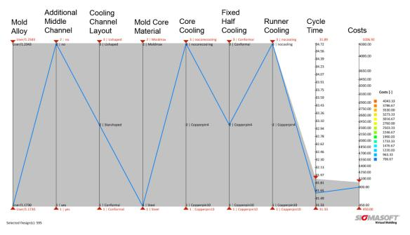
Figure 2 – In the assessment, it is easy to make further restrictions to the parameters and goals to find the optimum solution with low costs and a short cycle time
