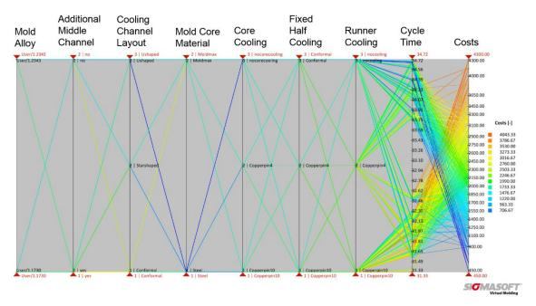
Figure 1 – With the new SIGMASOFT® Autonomous Optimization tool, the effect of cooling layout and alloy selection on cycle time and mold costs can be easily assessed. The image shows all possible combinations of mold and core alloys and cooling concepts for a thermoplastic part and their effect on mold costs.
