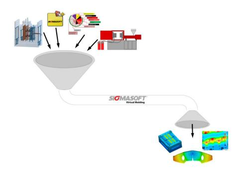
Figure 1 – With conventional approaches for injection molding simulation the user provides a combination of geometries, materials and process set-up and receives a result for this specific point inside the process window
