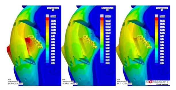
Figure 1 – Temperature distribution on the mold core for the initially planned common mold steel (left), as well as the core inserts out of CuBe B2 (middle) and Moldmax HH (right)
