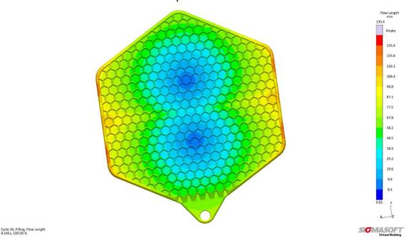
Figure 1 – A Flow length of 135 mm with a fine honeycomb structure and a wall thickness of 1 mm in the majority of the part – Interested visitors can experience the virtual as well as real production of the pot cloth at the booths of Momentive and SIGMA Engineering.
