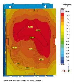
The reason for this varied outcomes is the temperature distribution inside the mold. While the classical approach assumes a homogenous temperature, the real mold shows quite high temperature variations. Taking a closer look on the moveable half after the thermal steady state is reached reveals that just inside the cavity the difference is already bigger than 30°C (Figure 4). The hot areas
