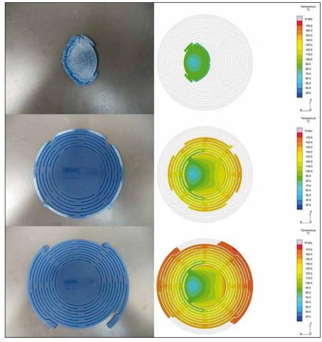
Figure 6: Comparison of short shots and simulation at 10 cm<sup>3</sup>, 40 cm<sup>3</sup> and 60 cm<sup>3</sup> (top to bottom).
