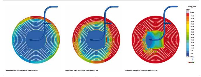
Figure 5: Curing degree at 25.5 s, 29.5 s and 35.5 s (from left to right) of the curing phase.
