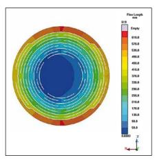
Figure 2: An interlaced geometry and a maximum flow length of 619 mm make the carry mesh challenging for production.
