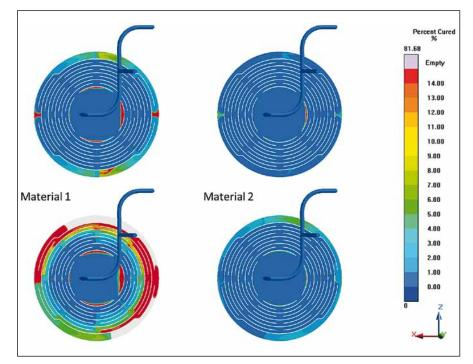
Figure 3: Evaluating the possibility to fill the part under the classical (top) and Virtual Molding approach (bottom) for materials one (left) and two (right).
