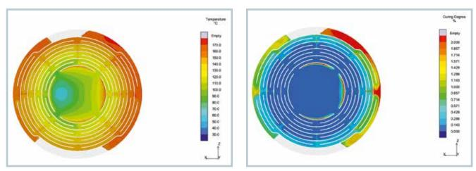
**Fig. 2.** Part filling of the LSR carry mesh: left the temperature distribution, on the right the curing degree both at around 93% filling level. The curing moves from the outside to the center of the part (figures: Sigma Engineering)
