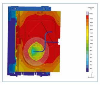
(Title figure), was evaluated with Sigmasoft Virtual Molding. The design article's labyrinthine geometry with a maximum flowlength of 619 mm requires stable flow and curing properties to guarantee a robust process and good part quality.
